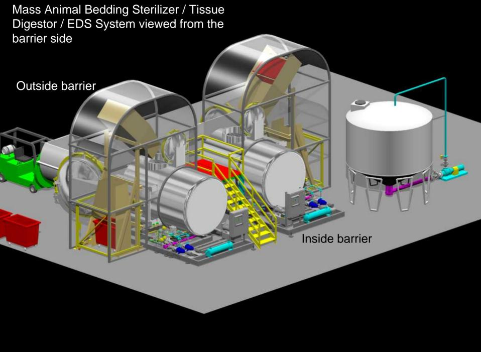
An EDS / Tissue Digestor can be substantially less expensive than a small EDS alone. This system is being built for Penn State University.
