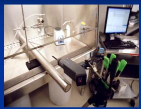
**Tracer Gas:** SF<sub>6</sub> ~ 10,000 ppm @ 20 psi through NSF 6-jet collision nebulizer w/H<sub>2</sub>O
